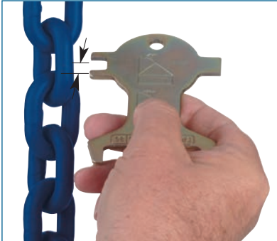
Inspection of material diameter
