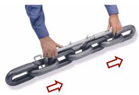
While the gauge legs have firm contact with the chain link roundings the relevant measuring value can be read on the scale (mm graduations).
