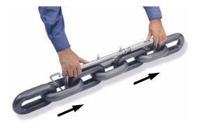
In addition to performing measurements with the chain gauge users can also send sections of chain (7 links, no adapter chains) to THIELE for testing. These samples must have completed the same number of operating hours as the rest of the chain. The test program includes various measurements, breaking-force tests and an assessment of fatigue and corrosion.
