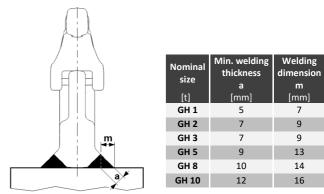
The weld seam must be led completely all around the weld-on hook.
