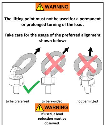
Please note that the values for the Working Load Limits as a function of number of legs and inclination angle given in Table 4 base on the preferred alignment.
