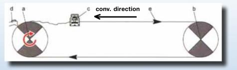
a) main drive b) tail-end drive c) chain securing device d) pawl e) conveyor direction during chain tensioning
