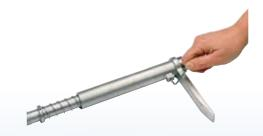
A grubscrew is used to prevent the sliding arm with scale from rotating. This grubscrew must not be fully tightened!
