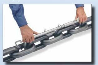
The measurement is then read off on the millimetre scale while the arms of the gauge are kept in contact with the respective links.
