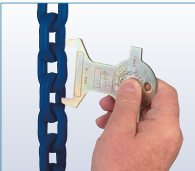
Inspection of permanent elongation
