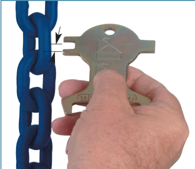
Inspection of material diameter
